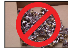
INCORRECT (Stored loose in a box)
